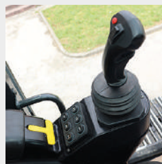
Control joystick for operating functions (left)
