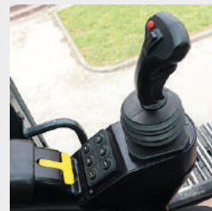
Control joystick for operating functions (left)
