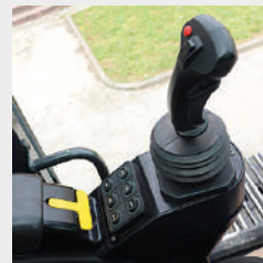
Control joystick for operating functions (left)
